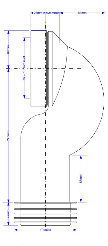
\*WC-INLET Seal has been tested to EN681
