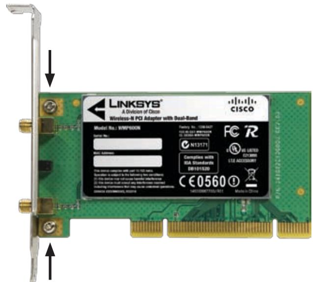
2. Use the two screws to attach the PCI board to the low-profile bracket.
