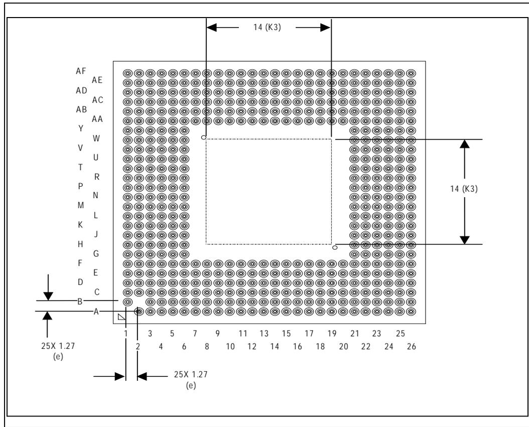
**NOTE:** All dimensions in millimeters. Values shown for reference only. Refer to [Table 4-1](#) for details.
