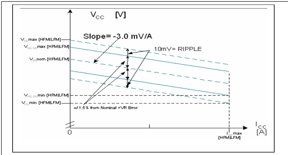
Figure 3-2. Deep Sleep VCC and ICC Load Line
