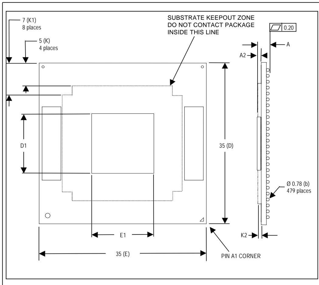
**NOTE:** Die is centered. All dimensions in millimeters. Values shown for reference only. Refer to [Table 4-2](#) for details.
