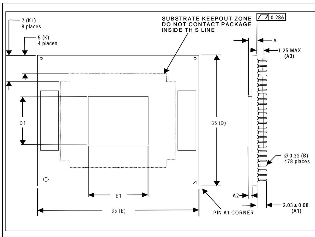
**NOTE:** Die is centered. All dimensions in millimeters. Values shown for reference only. Refer to [Table 4-1](#) for details.
